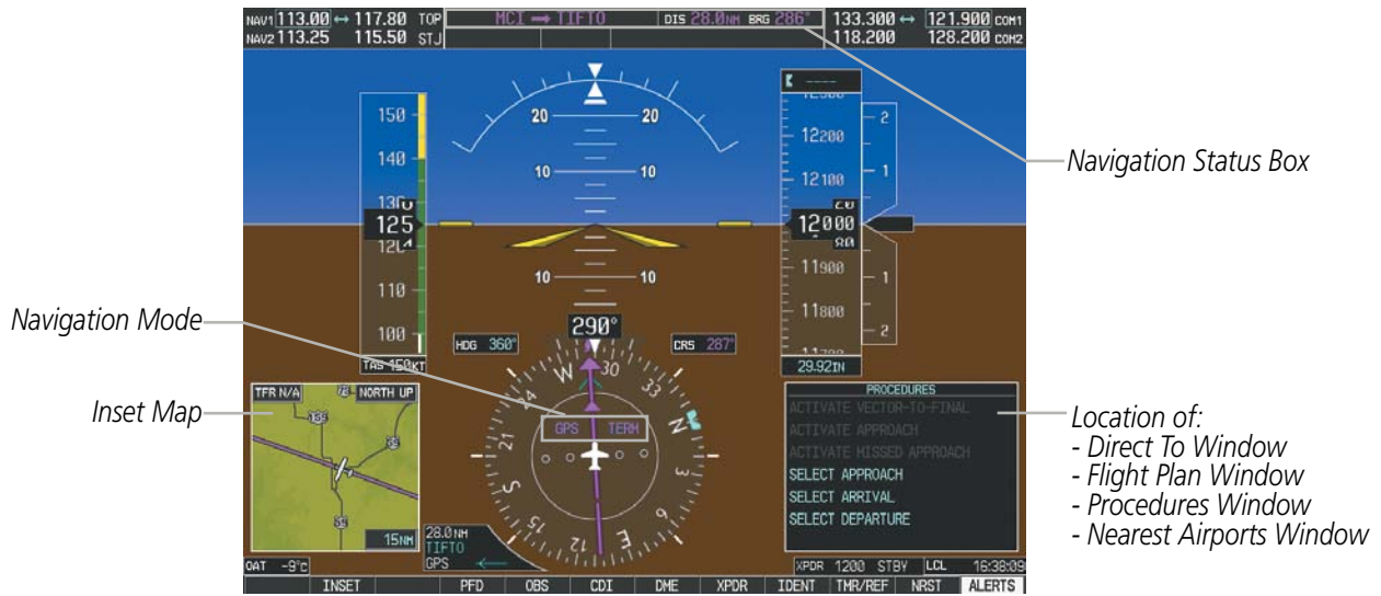
Figure 5-1 GPS Navigation Information on the PFD
