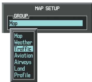
Figure 6-174 Navigation Map Page Setup Menu
