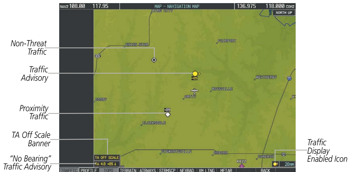
Figure 6-172 TAS Traffic on Navigation Map
