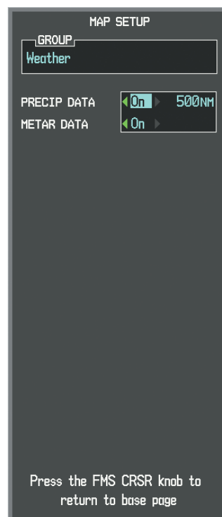
Figure 6-99 Navigation Map Page Setup Menu, Weather Group
