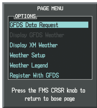
Figure 6-65 Weather Data Link (GFDS) Page Menu
