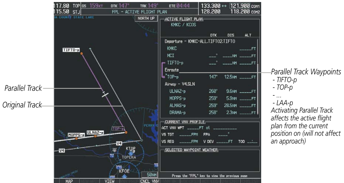
Figure 5-81 Parallel Track Active
