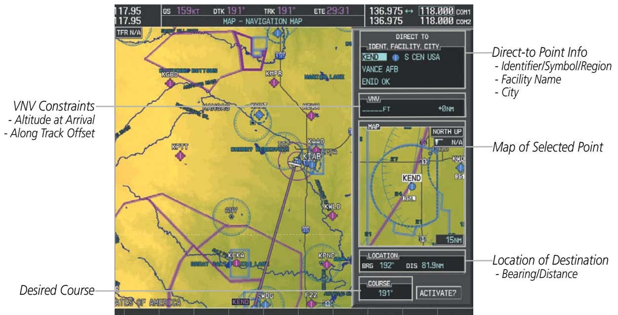
Figure 5-51 Direct-to Window - MFD
