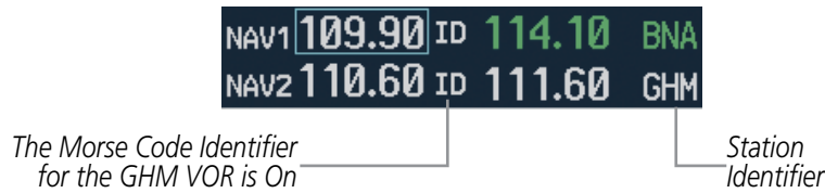
Figure 4-21 NAV Radio ID Indication
