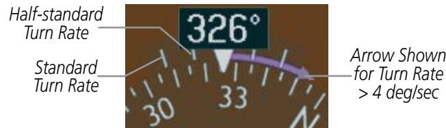
Figure 2-17 Turn Rate Indicator and Trend Vector
