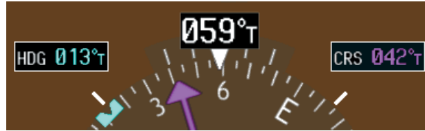
Figure 2-15 Heading and Course Indications (True)
