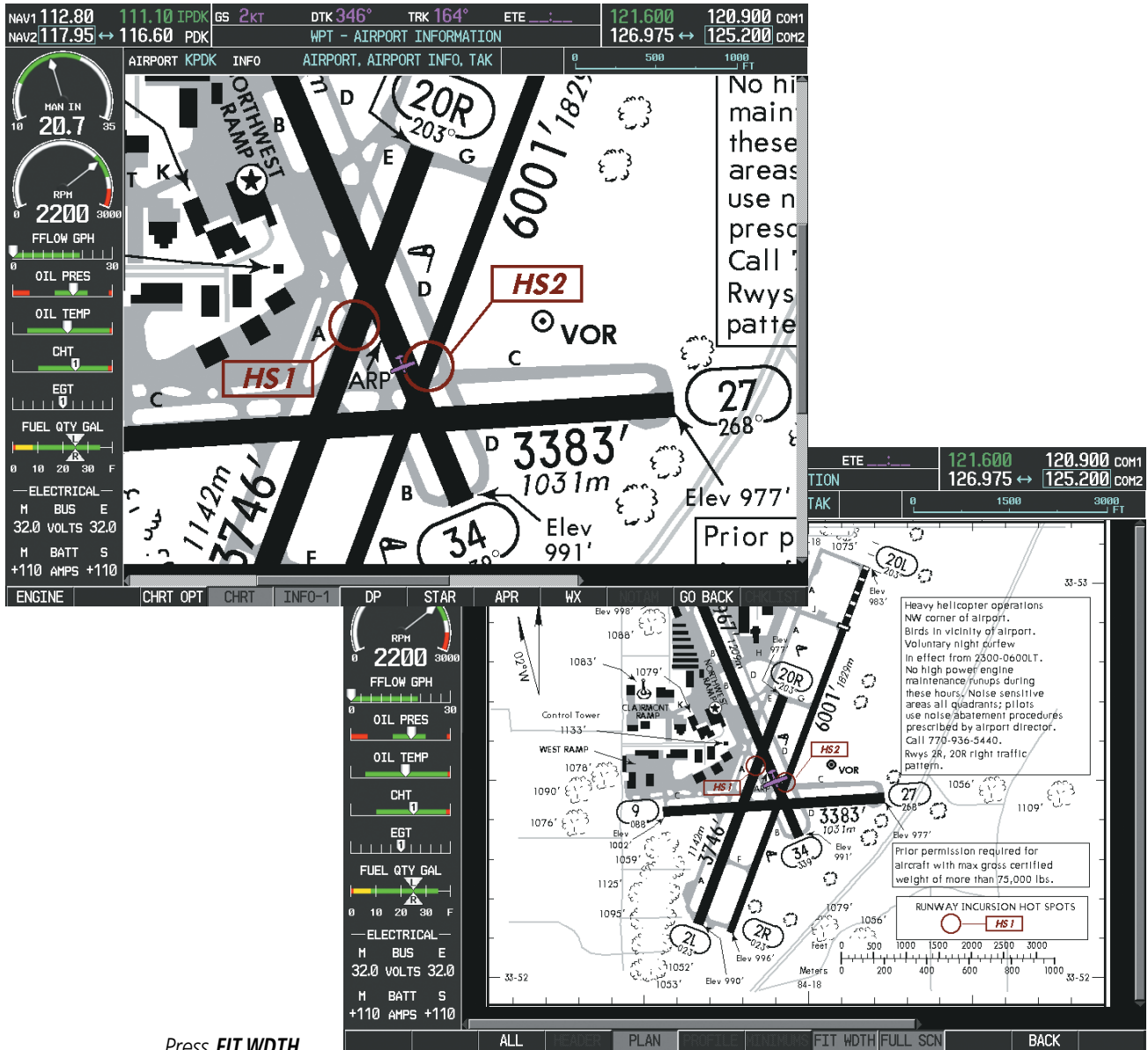
Figure 8-39 Airport Information Page, FIT WIDTH Softkey Selected
