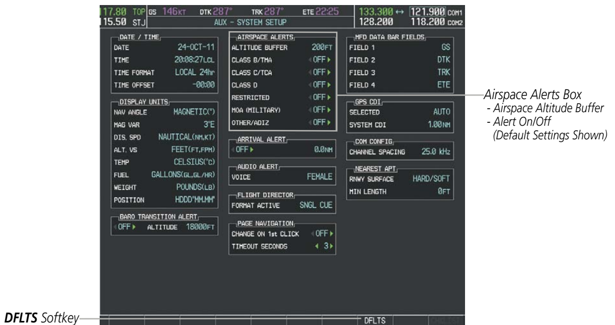
Figure 5-49 System Setup Page - Airspace Alerts
