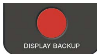
Figure 4-48 Display Backup Button
