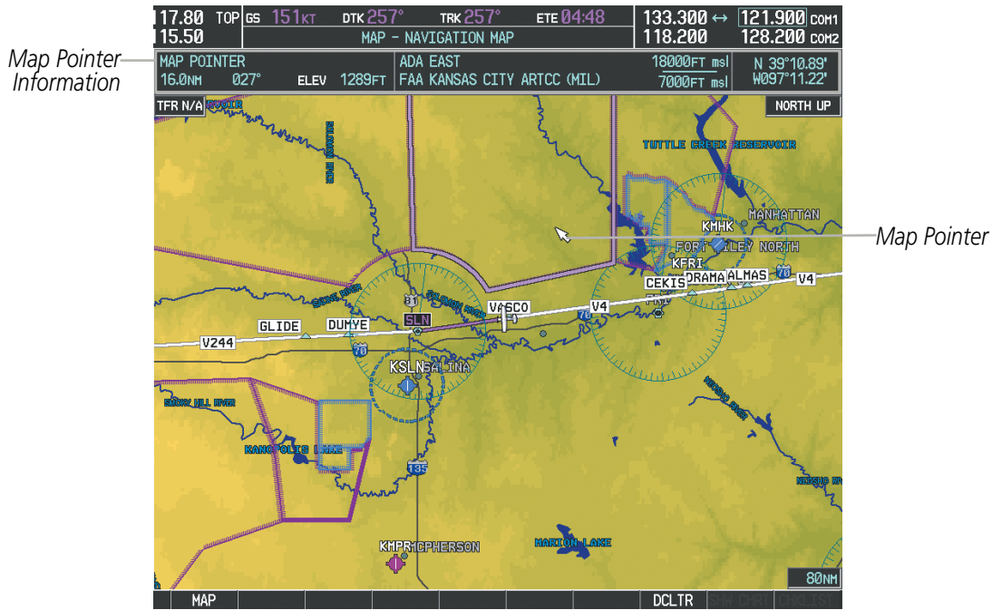
Figure 5-8 Navigation Map - Map Pointer Activated
