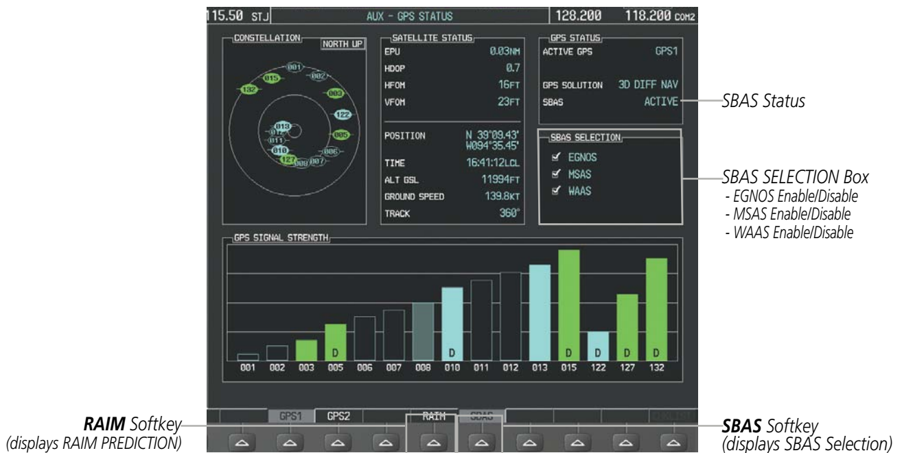
Figure 5-103 SBAS Display - Active
