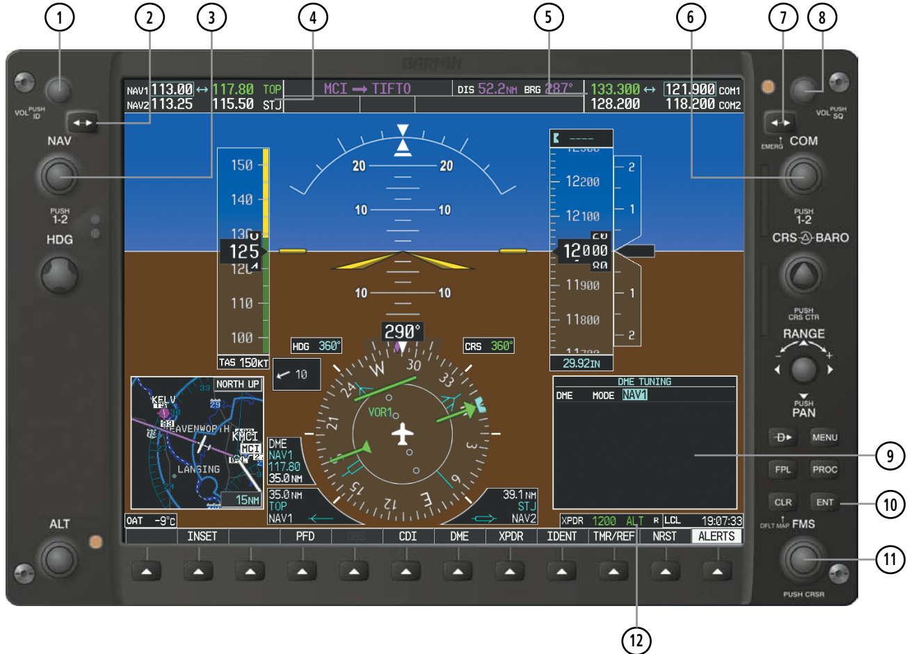
Figure 4-1 MFD/PFD Controls, COM/NAV Frequency Tuning Boxes, and DME Tuning Window (Cessna 172R PFD Shown)
