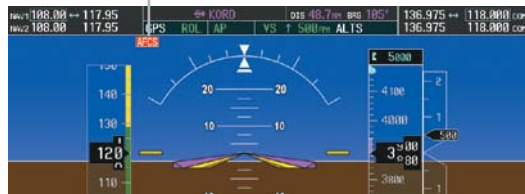
Figure A-6 AFCS System Status Field
