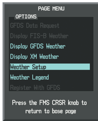
Figure 6-100 Weather Data Link Page (FIS-B) Menu
