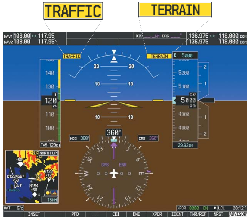
Figure 2-35 Traffic and TAWS Annunciations
