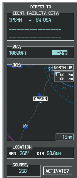
Figure 5-122 Enter VNV Offset Distance
