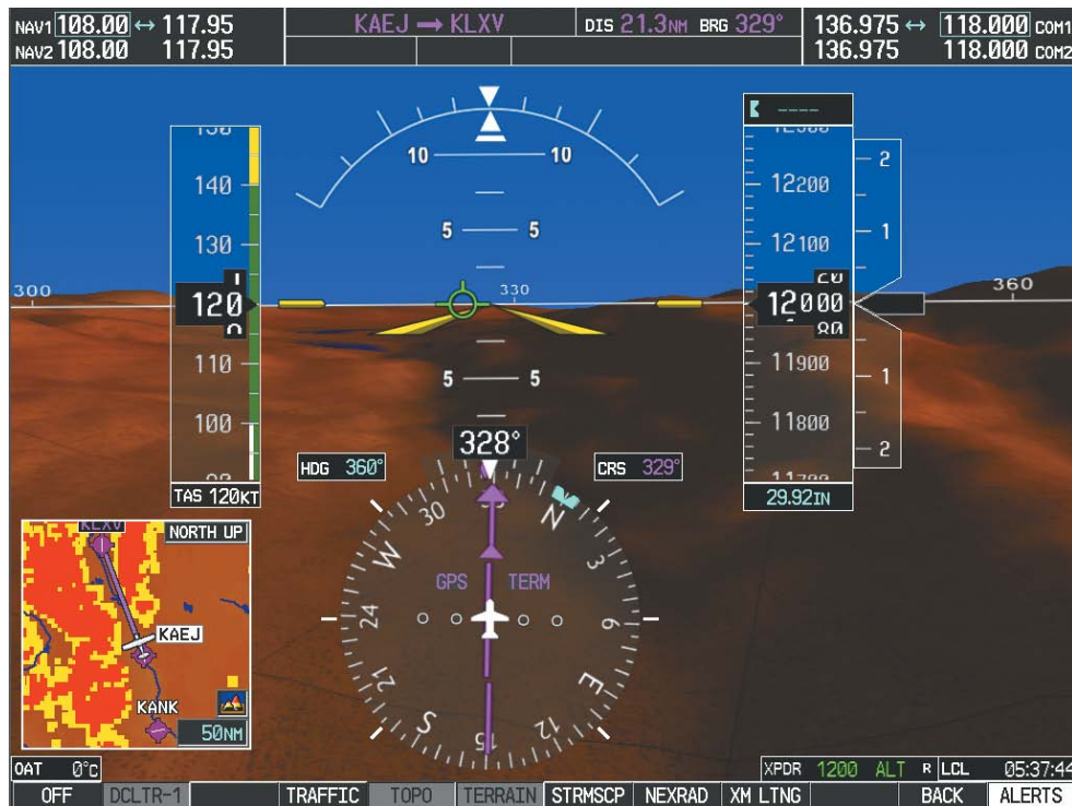
Figure 8-1 Synthetic Vision Imagery
