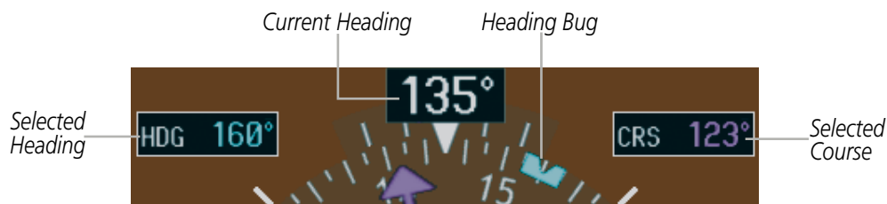
Figure 2-14 Heading and Course Indications (Magnetic)
